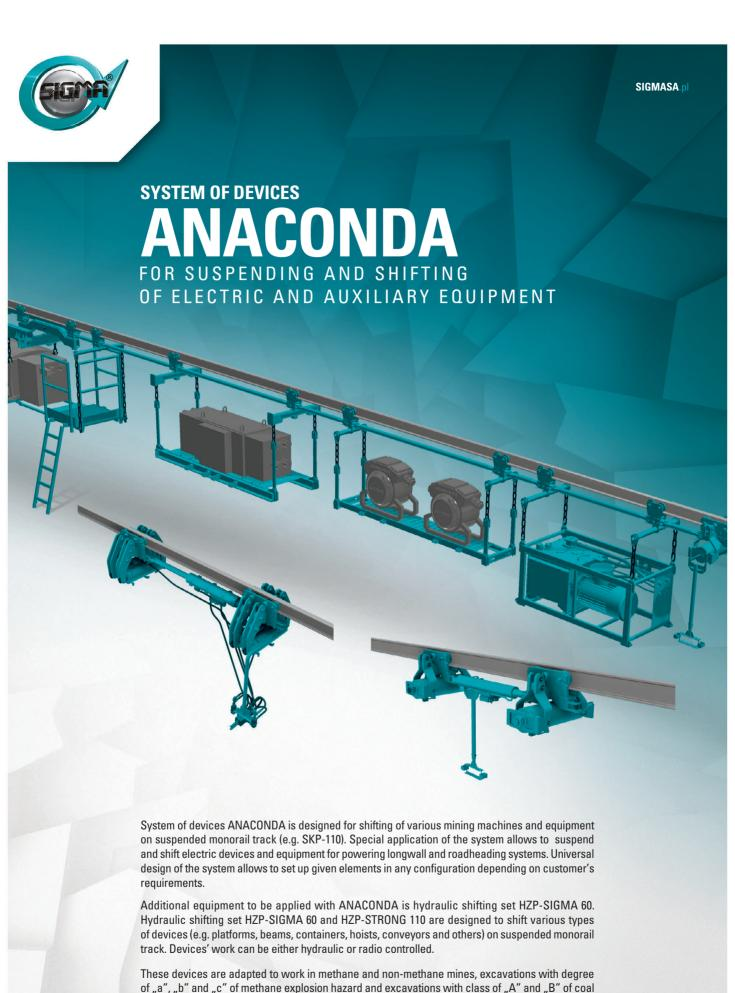
dust explosion hazard. This device has been classified as Group I, category M2 due to its application in areas exposed to danger of explosion (according to directive 2014/34/UE).
