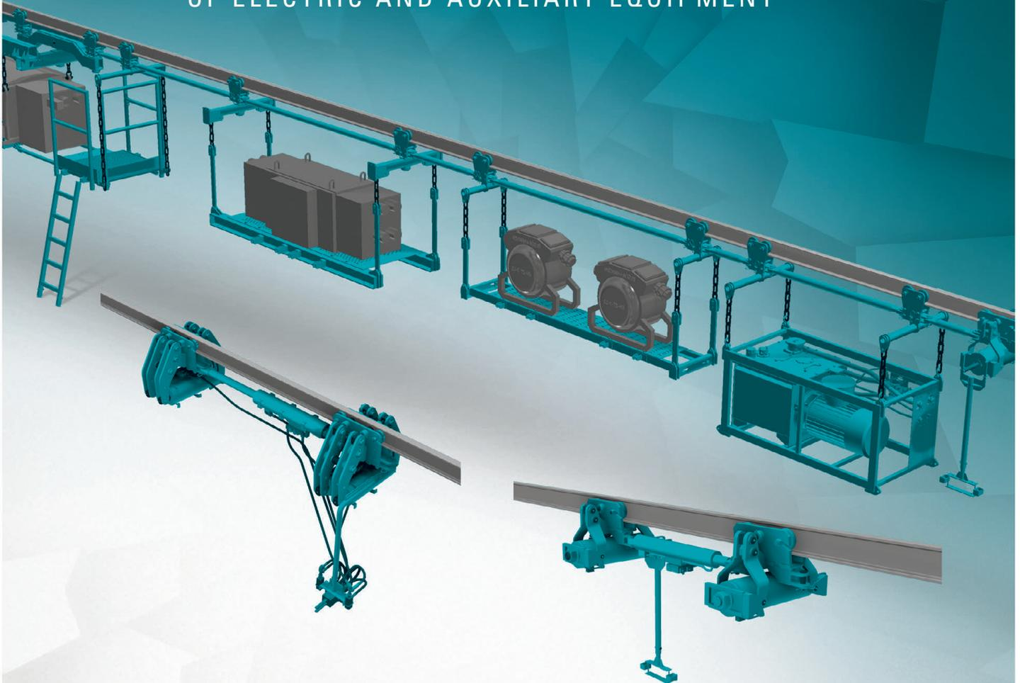
System of devices ANACONDA is designed for shifting of various mining machines and equipment on suspended monorail track (e.g. SKP-110). Special application of the system allows to suspend and shift electric devices and equipment for powering longwall and roadheading systems. Universal design of the system allows to set up given elements in any configuration depending on customer's requirements.
