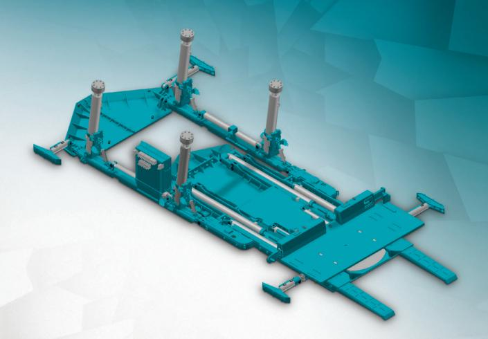
Powered roof support transportation and turning device OSS-ELEPHANT is applied to unload the powered roof supports from the rail, its turning and installation at longwall. The device can cooperate with both suspended monorail track or floor mounted rail.
