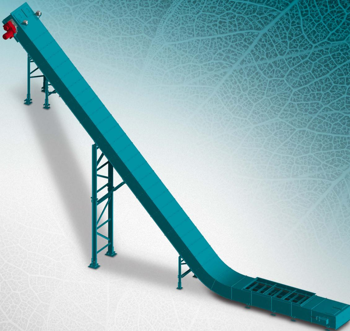
Scraper conveyors are designed to transport loose materials, both horizontally and at inclination angle up to 40°. They allow to transport input materials over long distances. Conveyor's size, as well as quantity and location of feed and discharge chutes (inlet and outlet channels) are adapted according to individual requirements of end user. One of the type of scraper conveyor in our offer is "redler" type conveyor.
