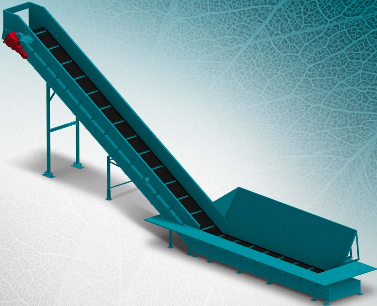
Chain conveyor belts are designed to transport various materials, including mixed municipal waste of heavy bulk load, as well as segregated light fractions like paper, plastic, foil. Due to its construction, chain conveyor belts can be bended in rising (incline) position what allows to transport input material to high located points, even in halls/buildings of limited spatial structure.
