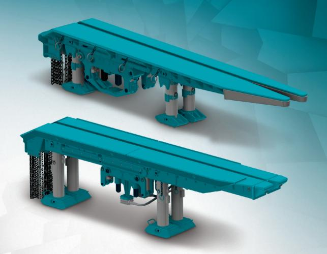
Prop and support devices PEGASUS and PEGASUS II are applied in order to assure proper support of roof in the area of crossing between longwall face and adjacent roadway. This is special type of support designed to build over the niche between last roof support and adjacent roadway.
