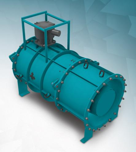
Axial flow fan WL-SIGMA 650 is designed for independent/separate ventilation of mining excavations (e.g. in coal mines, cooper mines). Axial flow fan WL-SIGMA 650 can operate as forcing fan, also as exhaust fan in auxiliary dedusting air-ducts or as forcing fan in auxiliary cooling air-ducts.
