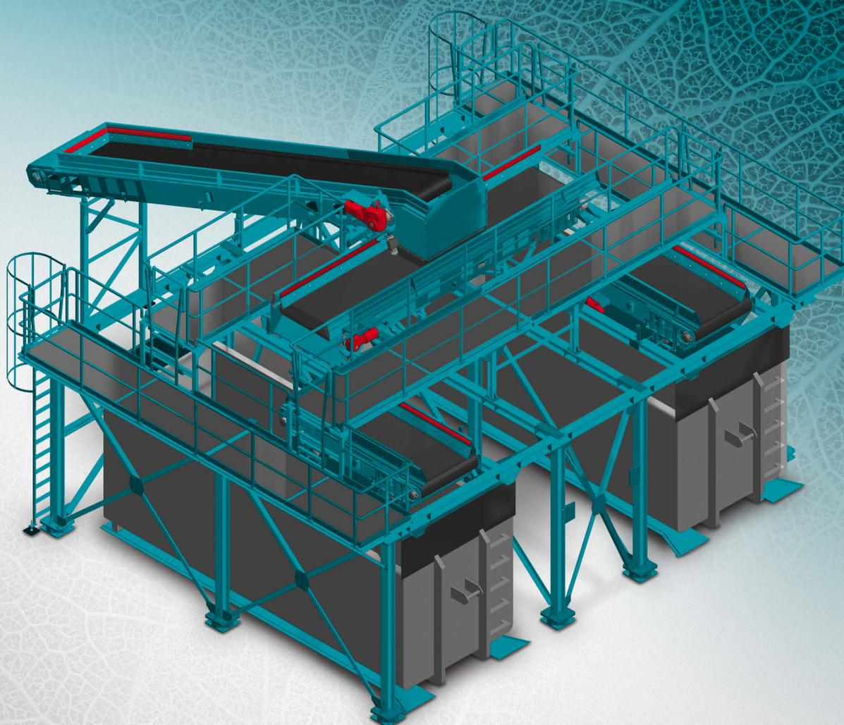
Automatic loading station enables the continuous filling in of containers and their replacement without necessity to stop (switch off) waste sorting line. Such loading (reloading) system ensures maximum possible filling in of container with input material. SIGMA S.A. offers two types of loading stations: with mobile passing loading conveyor and mobile rotation loading conveyor.
